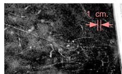
with the air filling the chamber, upon passing from right to left in the photograph. The most common mode of interaction under these conditions is Compton scattering.
